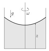
Figure 16: rotating fluid in a container.
