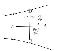
Figure 4: Physical meaning of vorticity.  $\boldsymbol{\omega}$  is taken to point out of the page. The angular velocity of the two perpendicular fluid element lines AB and CD is  $\partial_x v_y$  and  $-\partial_y v_x$  respectively. Hence their average angular velocity is  $(\partial_x v_y - \partial_y v_x)/2 = \omega/2$ .
