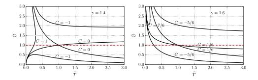
Figure 19: Solutions to equation (312) for different values of C. Left panel is for  $\gamma = 7/5$ , corresponding to a diatomic gas. Right panel is for  $\gamma = 1.6$ .
