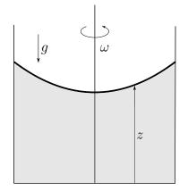
Figure 1: Rotating fluid in a container.
