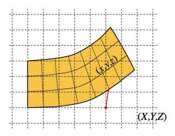
Figure 1.1: A picogram showing how the internal material coordinates (x, y, z) and the spatial coordinates (X, Y, Z) relate to each other in case of a material deformation.
