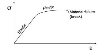
Figure 1.2: Stress response regimes of a solid material to an imposed strain.
