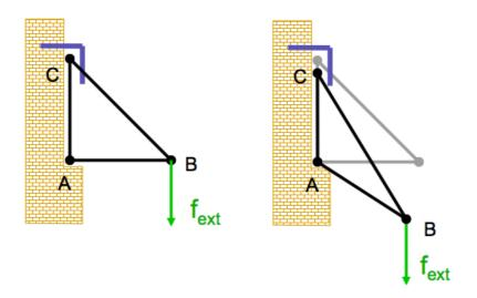
Figure 1.5: The static problem we wish to solve. Left: before application of force. Right: after application of force.
