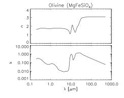
Material with n = 1 and k = 0 would be invisible, since it would have the same optical properties as vacuum. Typically n has values not much smaller than 1 and not much bigger than a few.
