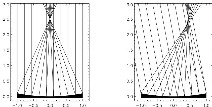
Figure 2.1: Results of a simple computation of ray reflection off a parabolic mirror with  $a = 0.1$  and hence  $f = 2.5$  for on-axis incident radiation (left) and off-axis incident radiation (right). The off-axis angle of incidence is 10 degrees.
