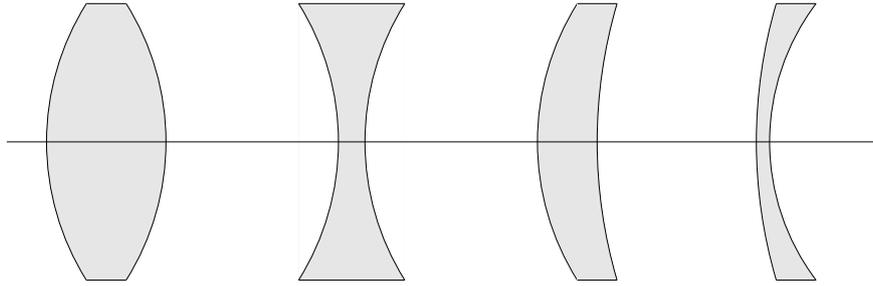
Figure 2.4: Some example shapes of lenses. From left to right: biconvex lens, biconcave lens, positive meniscus, negative meniscus.
