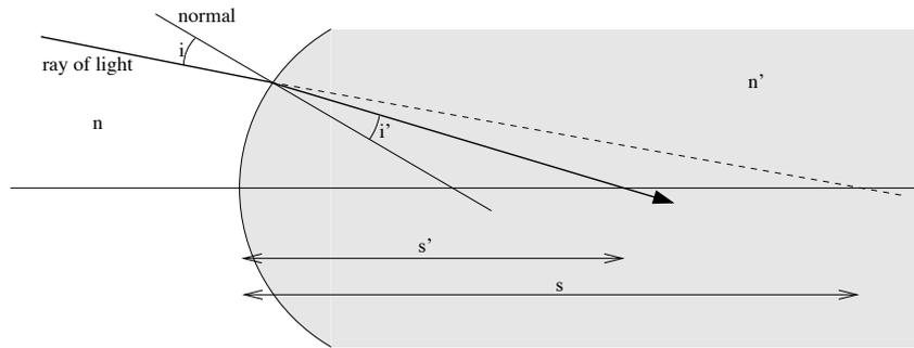
Figure 2.2: Refraction of light at a spherical interface between a medium of refractive index  $n$  (left) and a medium of larger refractive index  $n'$  (right).
