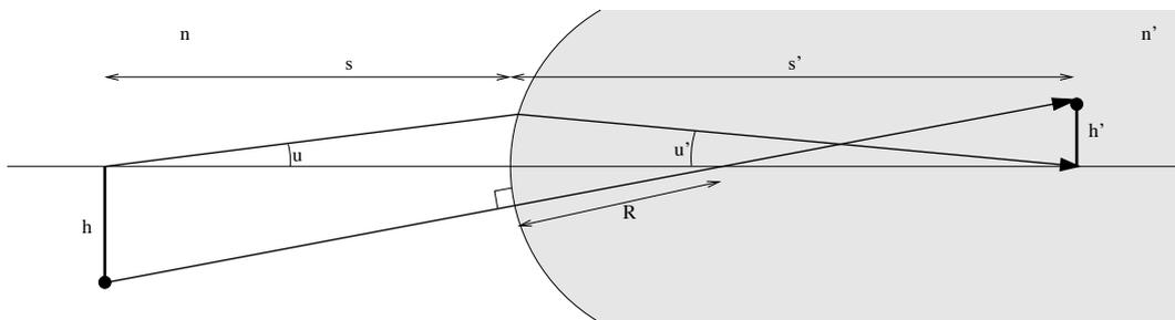
Figure 2.3: Same system as in Fig. 2.2, but now the case where the two conjugate points are on opposite sides of the spherical interface.
