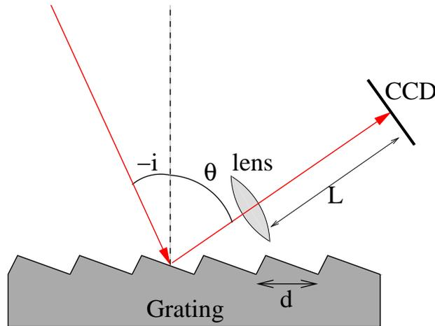
Figure 1: Schematic view of the setup of a grating with groove spacing  $d$  with incident radiation at an angle of  $i$ , and a CCD chip at angle  $\theta$ , with a lens of focal length  $L$  between the CCD chip and the grating to focus the light onto the CCD.
